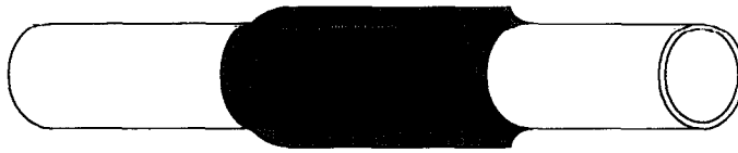
Fig. 5. Schematic of pipes or tubing connected by a shape memory alloy ring.
